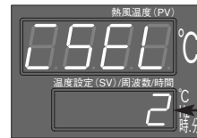
"2": to control with thermocouples of in put of thermocouples-2 of outer control terminal.
