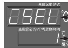
in put of thermocouples for control a code indicated. "1": to control with thermocouples assembled in device.
