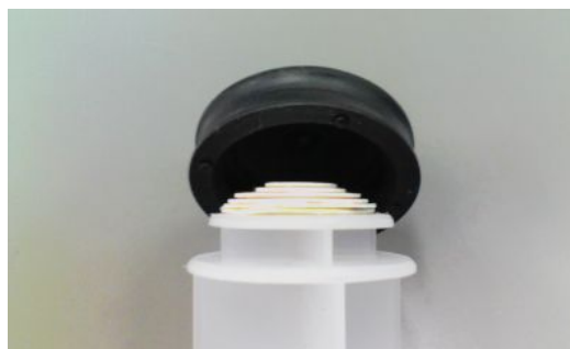
Fig.3.2.4 Remodeling of piston top
