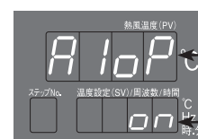
Self-holding setting of Temperature Control Error 1 Corresponds to internal air outlet thermocouple Self-holding with "on"
