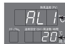
Temperature Control Error 1 trigger value settings Corresponds to the internal air outlet thermocouple Default value "20"
