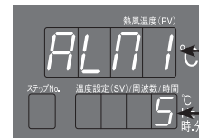
Temperature Control Error 1 alarm type: Corresponds to the internal air outlet thermocouple Upper deviation limit alarm with "5"
