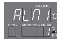
Change the set value to "1" to set the alarm to absolute upper limit
