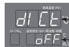
External temperature control enable setting code
