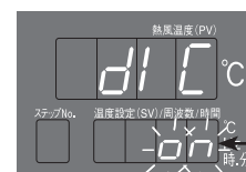
Use the ▲ key to switch to "on" and it will blink (waiting for confirmation)
